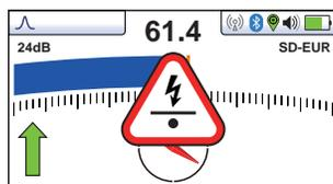
Real-time warnings are displayed across the receiver's display and accompanied by a mechanical vibration alert. Warnings are logged along with the cover of depth information when using the data logging feature of the receiver. All warnings can be turned on or off through the receiver's setup menu.
