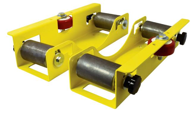
The SMP-RP-MPX reel roller system is ideal for storage, dispensing and management solution of cable reels ranging from 12" to 30" in diameter. The SMP-RP-MPX is sold in pairs and can accommodate cable drums with weights up to 750 pounds. The ten (10) gauge steel frames include three (3) position adjustments for the rollers, carrying handles for easy transport and pre-drilled holes for permanent mounting applications.
