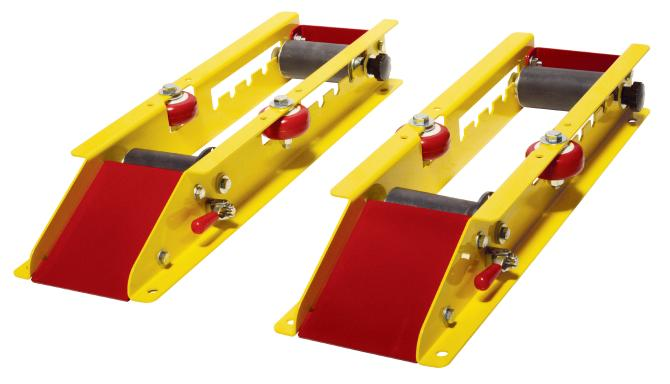
The SMP-RP-HDX reel roller system is ideal for storage, dispensing and management solution of cable reels ranging from 12" to 48" in diameter. The SMP-RP-HDX is sold in pairs and can accommodate cable drums with weights up to 3,000 pounds. The ten (10) gauge steel frames include five (5) position adjustments for the rollers, a slanted loading ramp, front roller locks for easy loading & unloading, and pre-drilled holes for permanent mounting applications.
