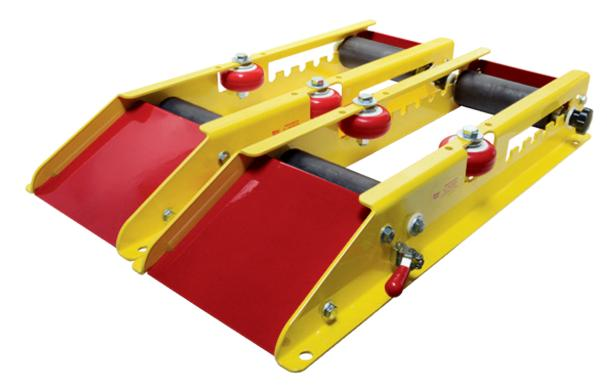
The SMP-RP-6K reel roller system is ideal for storage, dispensing and management solution of cable reels ranging from 12" to 48" in diameter. The SMP-RP-6K is sold in pairs and can accommodate cable drums with weights up to 6,000 pounds. The seven gauge steel frames include six (6) position adjustments for the rollers, a slanted loading ramp, front roller locks for easy loading & unloading, and pre-drilled holes for permanent mounting applications.
