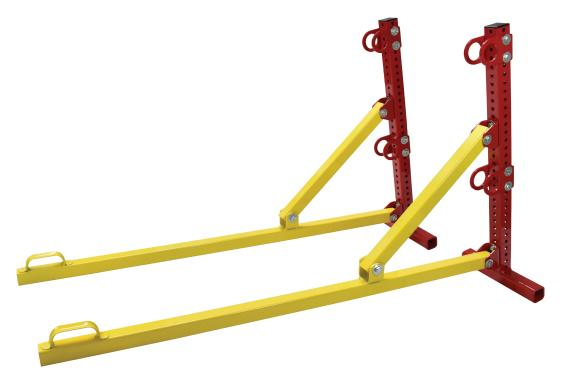
The SMP-LJ-54 cable reel jack is a quick & economical way to set-up reels of strand or cable. This versatile tool can be used on the ground, in a truck or on a warehouse floor. Constructed from heavy-wall square steel tubing, this labor saving tool will easily lift reels up to 54" in diameter. The lever action reel jack features adjustable arbor positions for reels of varying diameters, welded construction and a powder coated finish. Arbor spindle pipe not included.
