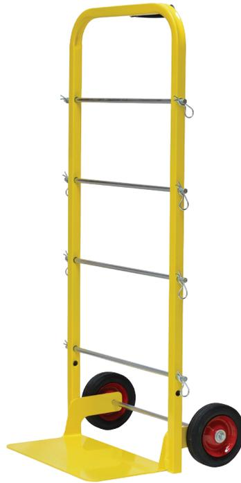
The SMP-HTC versatile and rugged wire cart dolly is designed for years of reliable in-field service. Constructed from welded steel tubing, this heavy duty cart can carry and dispense any spooled product that does not exceed 17" wide x 16" diameter. The wire cart features four (4) 0.5" solid steel spool bars (zinc plated for corrosion resistance), 6" solid rubber tires, a heavy-duty handle and a toe plate for use as a hand truck.
