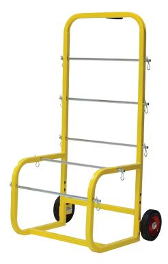
The SMP-CC versatile and rugged wire cart is designed for years of reliable in-field service. Constructed from welded steel tubing, this heavy duty cart can carry and dispense almost any spooled product that does not exceed 16" diameter. The wire cart features 6" solid rubber tires, a heavy-duty handle, and five (5) 0.5" solid steel spool bars (zinc plated for corrosion resistance) that can be removed to allow support for additional 16" diameter spools.
