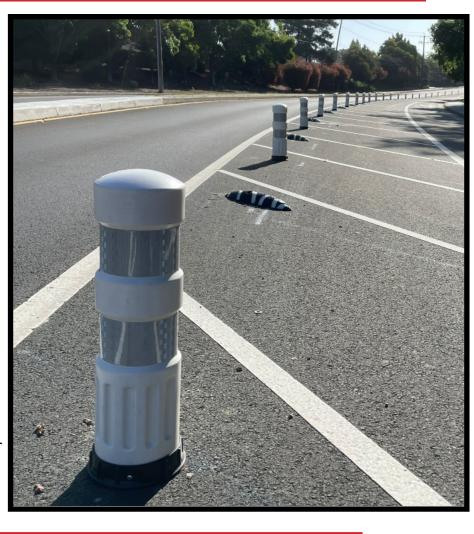
TD5428M is designed to replace other manufacturer's bollards that use metric thread anchors, with M12-1.75 threads. Before installing please clean out the existing anchor hole of any dirt or debris. It is also recommended to coat the threads with a moisture-displacing grease that will prevent galvanic corrosion, common to metalic anchors.
