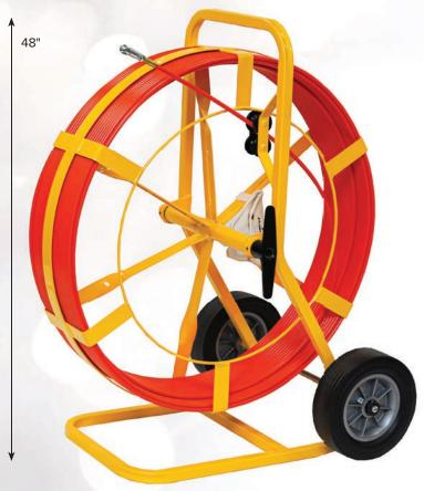
The Mega Buddy® features 1,500' rod and all-terrain wheels for longer cable pulls. Heavy duty non-conductive rodder for conduit 4" or larger to use manhole-to-manhole work or long-run cable pulls. Utilizing the Big Buddy® frame, the Mega Buddy® has the versatility to handle the toughest jobs. For conduit 4" or larger diameter.
