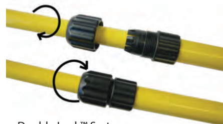
Double Lock™ System Extend pole sections to desired length, twist top pole to engage internal lock then tighten outer cap lock to secure.
