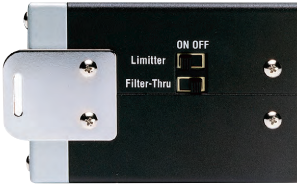
Figure 3-4 Limiter and Filter-Thru Switches
