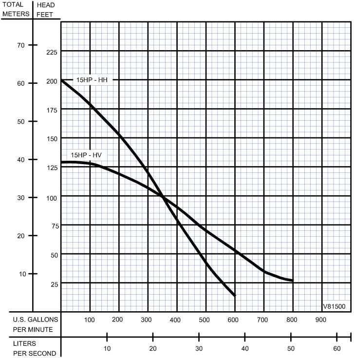
Testing is performed with water, specific gravity 1.0 @ 68° F @ (20°C), other fluids may vary performance
