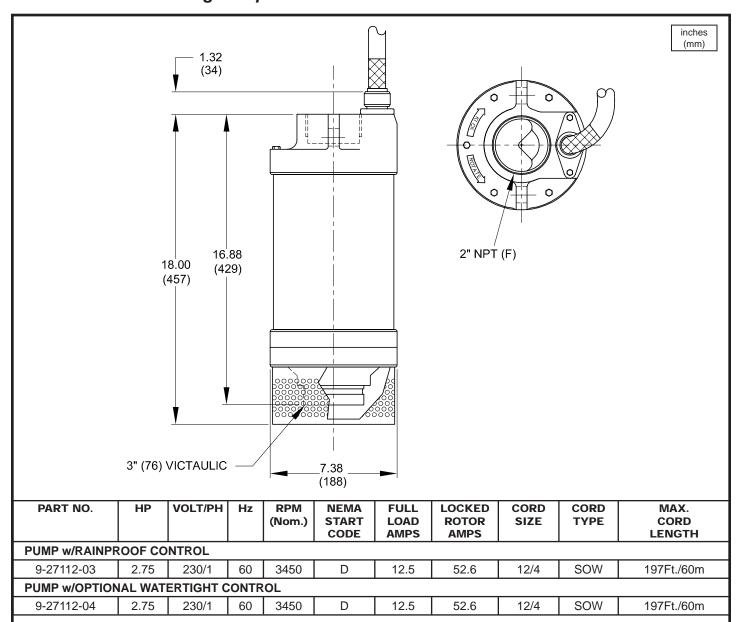
Pump rated for operation at  $\pm$  10% voltage at motor.
