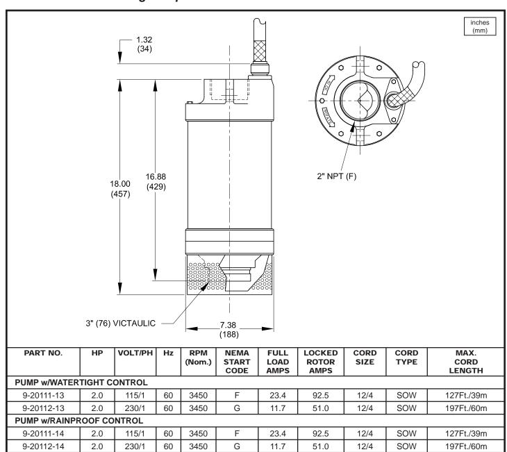
Pump rated for operation at ± 10% voltage at motor.
